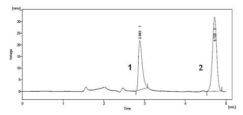
**Figure 5.** Chromatogram of boswellic acid (1) and myristicin (2) by HPLC with UV-VIS detection. Reprinted with permission from the Authors [52].
