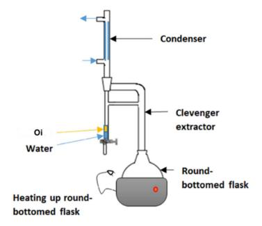
**Figure 4.** Clevenger apparatus used for hydrodistillation. Reprinted with permission from the Authors [47].
