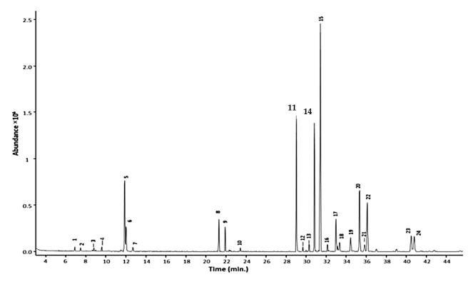
**Figure 2.** GC chromatogram of Ocimum micranthum Willd leaves' essential oil obtained with a capillary column coated with a mid-polar stationary phase 50%-phenyl-methylpolysiloxane. Peaks: eugenol (11); methyleugenol (14). Reprinted with permission from the Authors [21].
