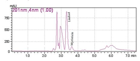
**Figure 6.** Chromatogram of myristicin and linalool in a plant by HPLC with DAD. Reprinted with permission from the Authors [53].
