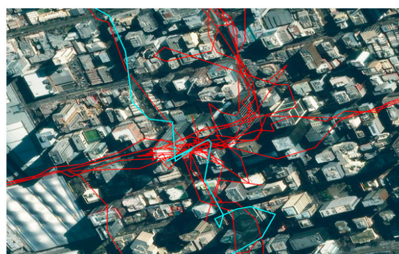
(b) Cycling tracks with location imprecisions due to urban canyon and GPS drift in intersections
