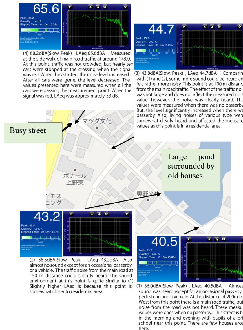
Figure 5. Example of sound map with Leq(A) (30 sec, Signal Scope Pro 7 on iPhone 5s), and sound spectrum (bs-spectrum on iPhone 5s): Ueno-higashi area, Toyonaka City, Osaka, Japan.
