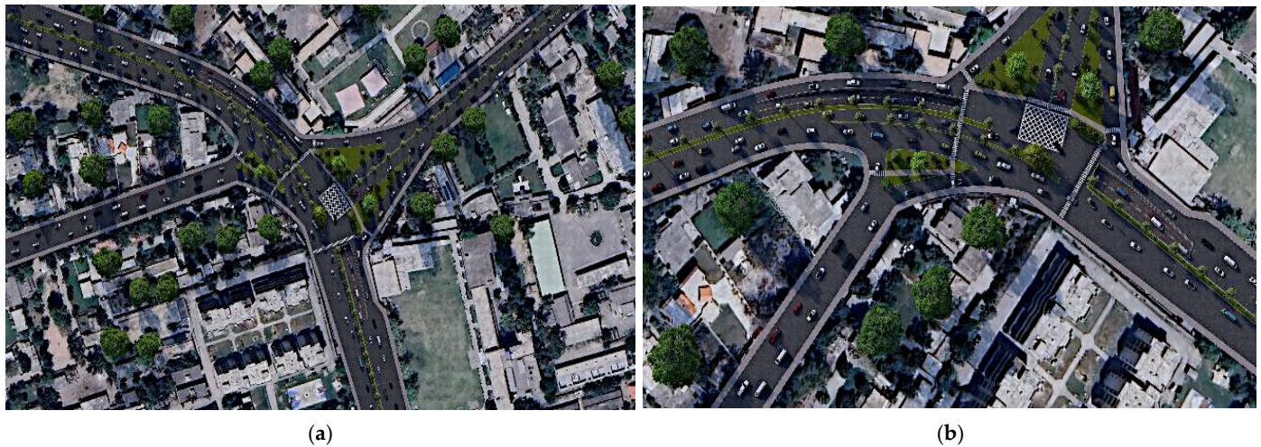
Figure 14. Proposed Grade Separation at Chungi Chowk: (a) Macro-level aerial layout of the intersection corridor and (b) close-up view of geometric interventions and traffic channelization.
