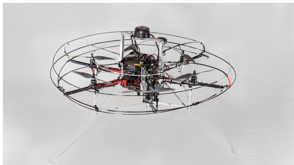
Figure 3. The hexacopter used for the real-life experiment is equipped with a RPLidar A2M4 laser scanner on top to sense its surroundings. There is a laser altimeter mounted at the bottom to sense the altitude of the UAV. The small Intel UPBoard and the Pixhawk autopilot are mounted below the laser scanner near the vehicle’s center of gravity.
