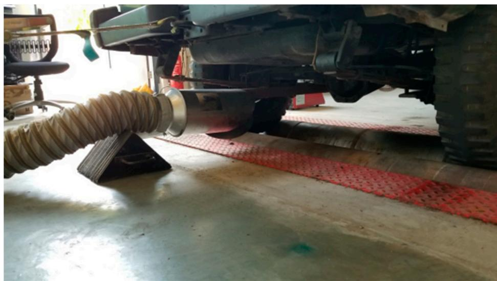
**Figure 4.** Vehicle exhaust removal system and rollers of the chassis dyno.
