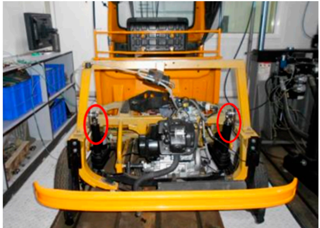
Figure 29. Experimental setup implementing an automated actuator control system marked in red circle.
