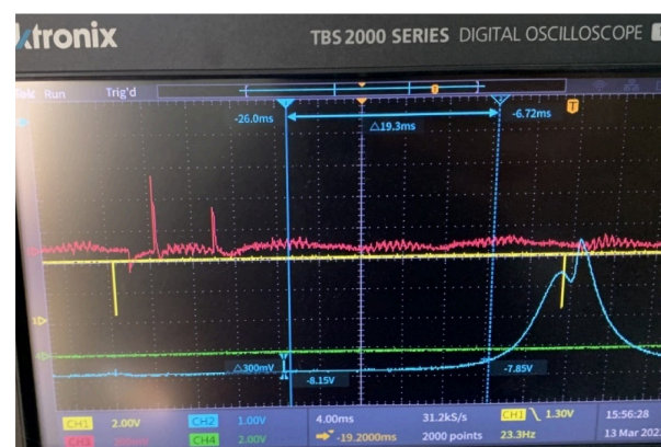
Figure 2. Ammonia injection signals and in-cylinder pressure trace.
