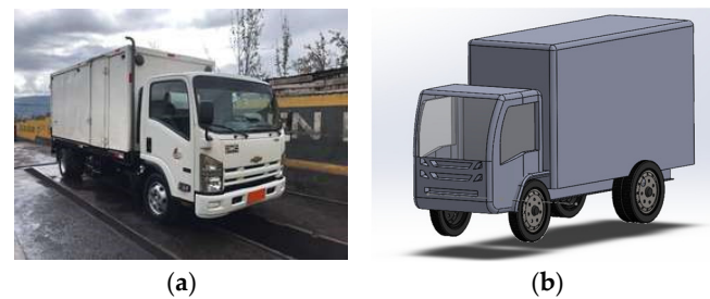
Figure 2. (a) Baseline vehicle configuration considered in this study; (b) simplified CAD model used for numerical analysis.
