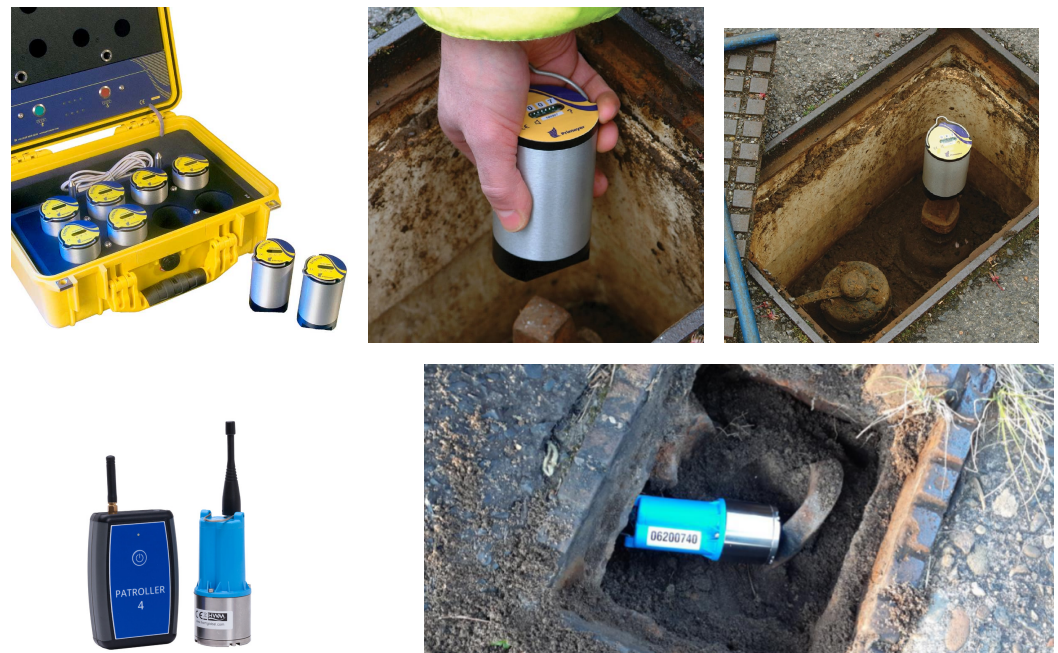
Figure 1. Primayer Enigma (top) and HWM PCorr+ (bottom) L&S correlating vibro-acoustic sensors.
