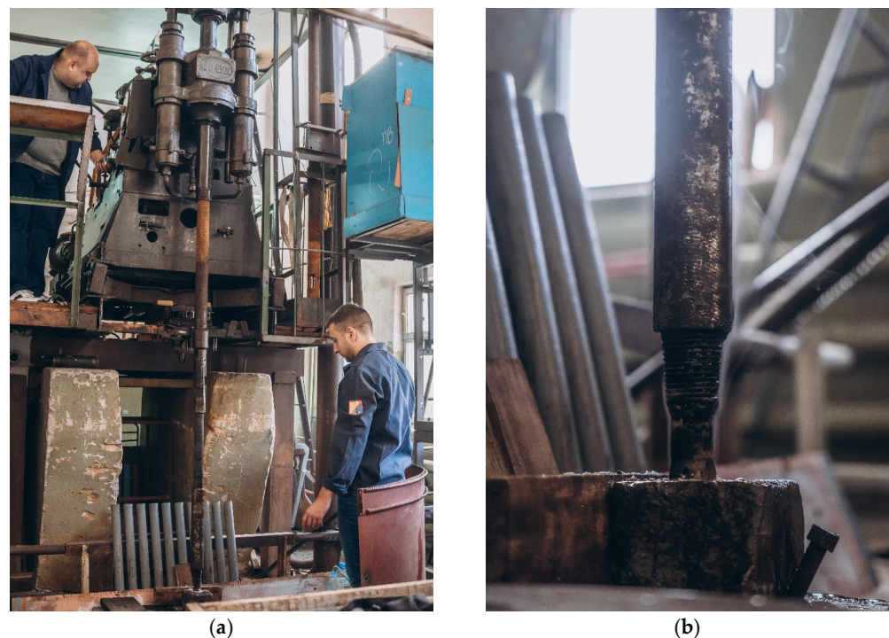
Figure 3. Photograph of the experimental setup. (a) Overall view of the drilling stand; (b) close-up of the instrumented tool holder.
