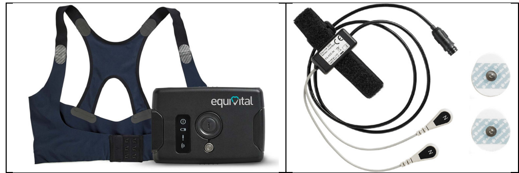
Figure 2. Equivital device (Equivital, Cambridge, UK) ( Left: Torso belt with sensor for HR and BR; Right: GSR sensors).
