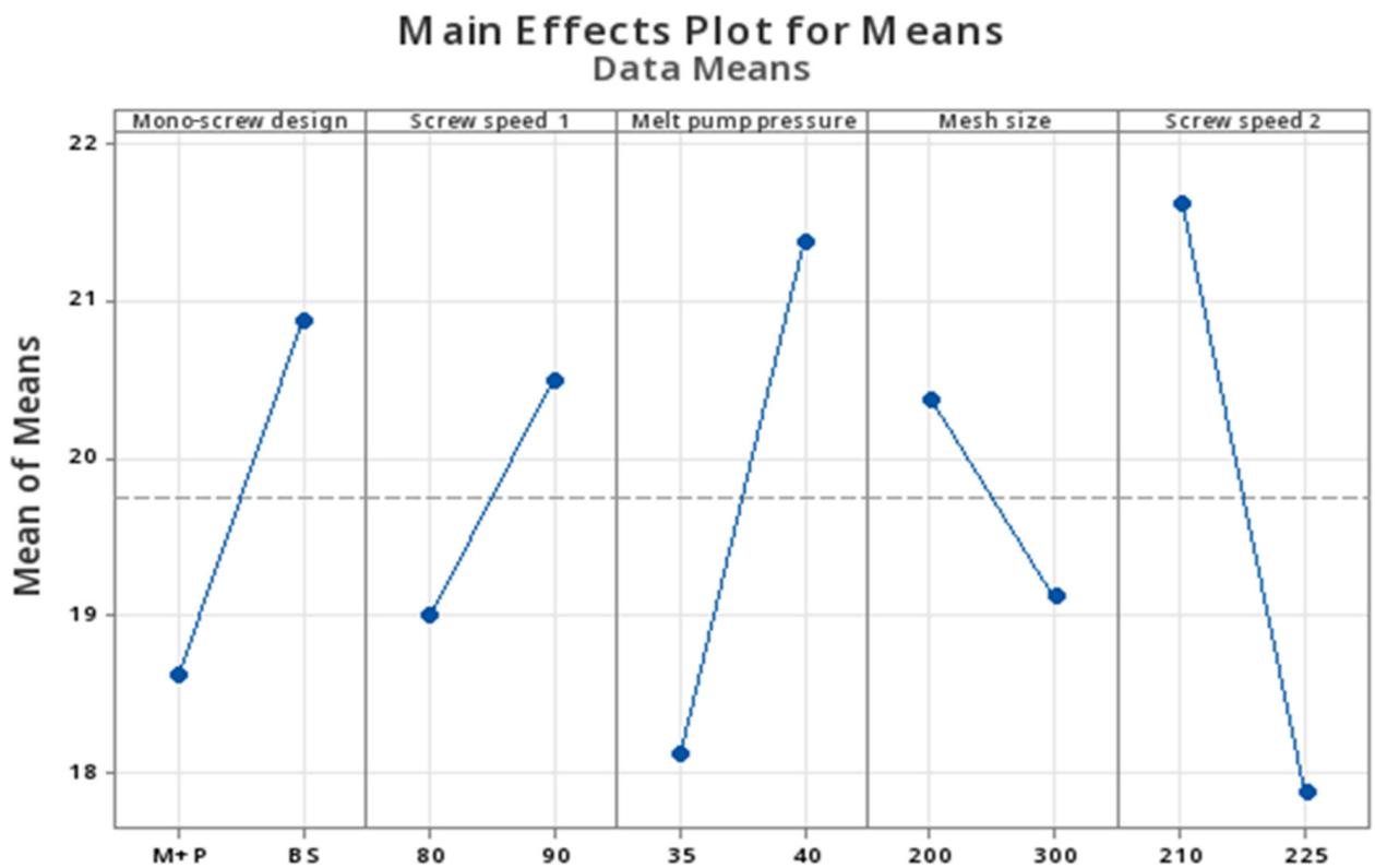
Figure 9. The gain of flexural modulus (%) vs. line's parameters.
