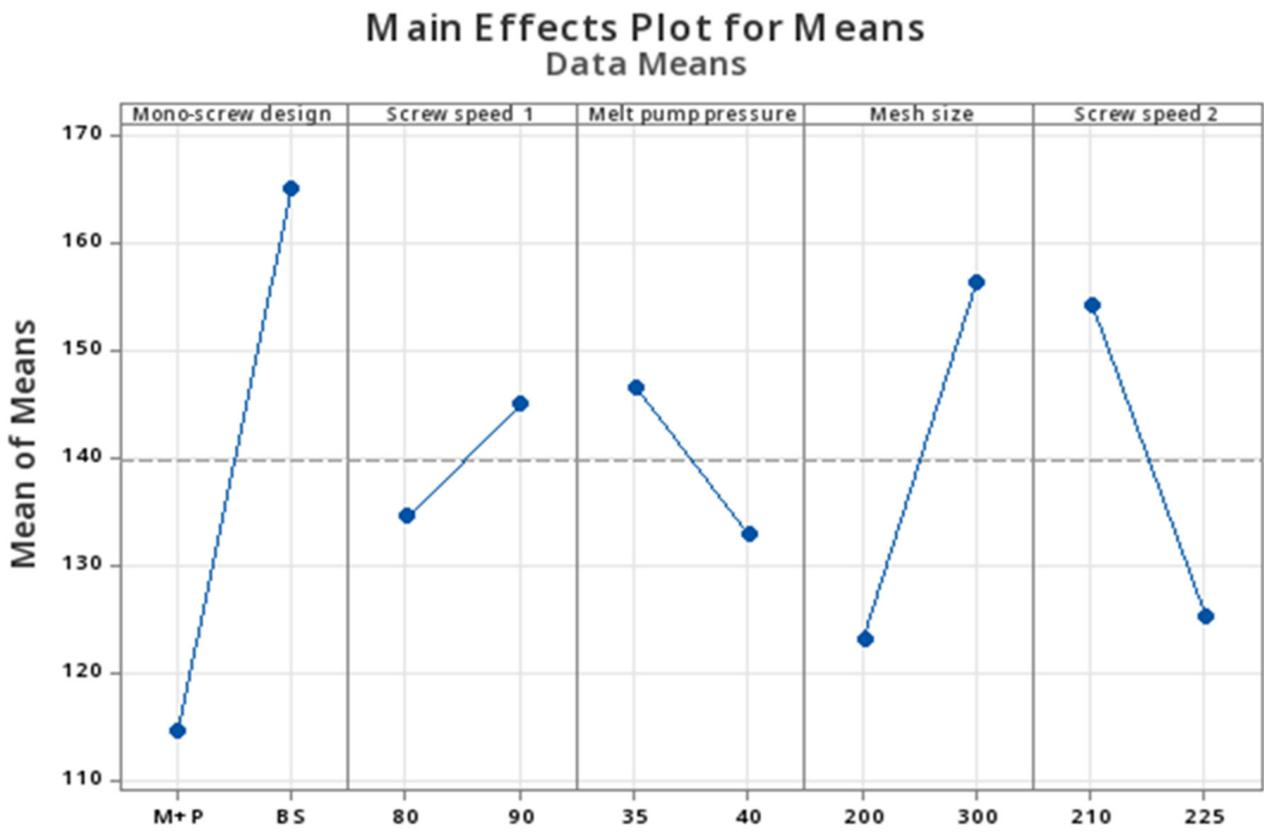
Figure 8. The gain of elongation at break (%) vs. line's parameters.
