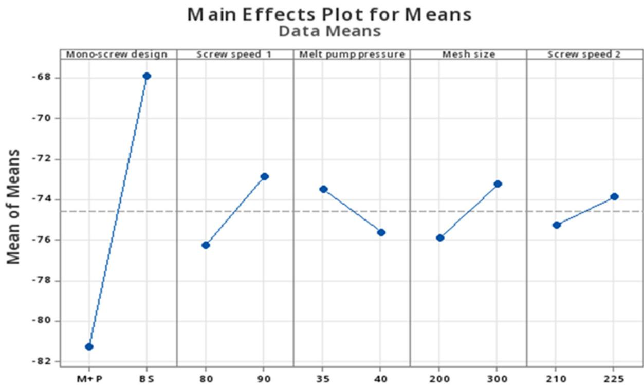
Figure 7. The gain of stress crack resistance (%) vs. line’s parameters.
