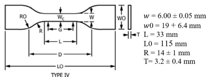
**Figure 3.** Dimensions of tensile test's specimen [19].
