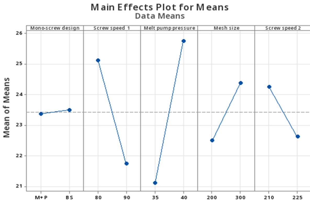
**Figure 10.** The gain of Izod impact strength (%) vs. line's parameters.
