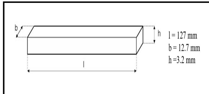
Figure 4. Dimensions of bending test's specimen [20].
