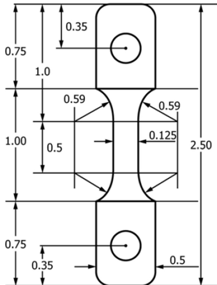
**Figure 6.** NCLS's specimen geometry [22].
