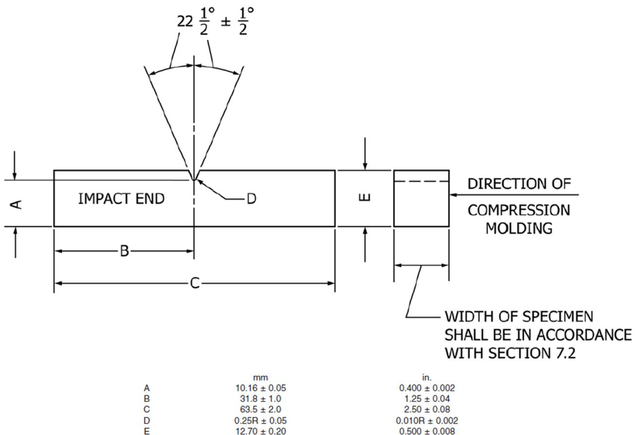
Figure 5. Dimensions of Izod type test specimen [21].
