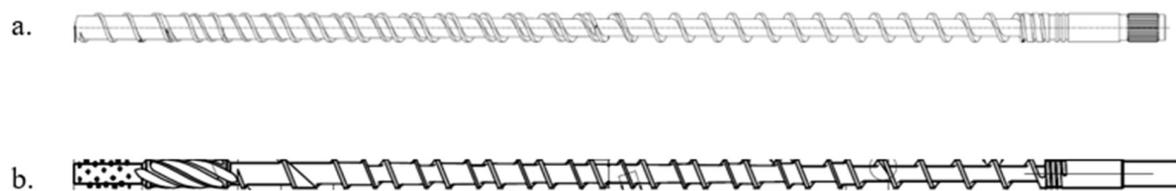
**Figure 2.** (a) Barrier screw (b) Screw with Maddock and pineapple.
