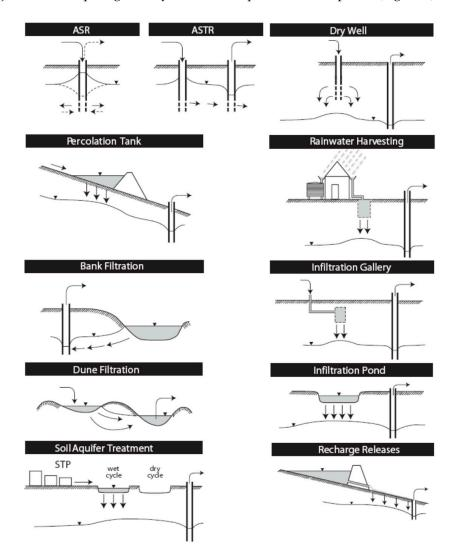
**Figure 1.** Schematic of types of MAR suited to urban water management (modified from: Dillon, 2005 [2]). ASR—Aquifer Storage and Recovery; ASTR—Aquifer Storage Transfer Recovery; STP—Sewerage Treatment Plant.
