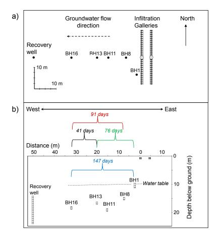
**Figure 3.** Residence time estimates between several boreholes (BH), using source water temperature as a tracer from a MAR infiltration gallery site (after Bekele et al., 2014 [38]). (**a**) in map view; (**b**) and relative to the maximum height of the water table in cross-section.
