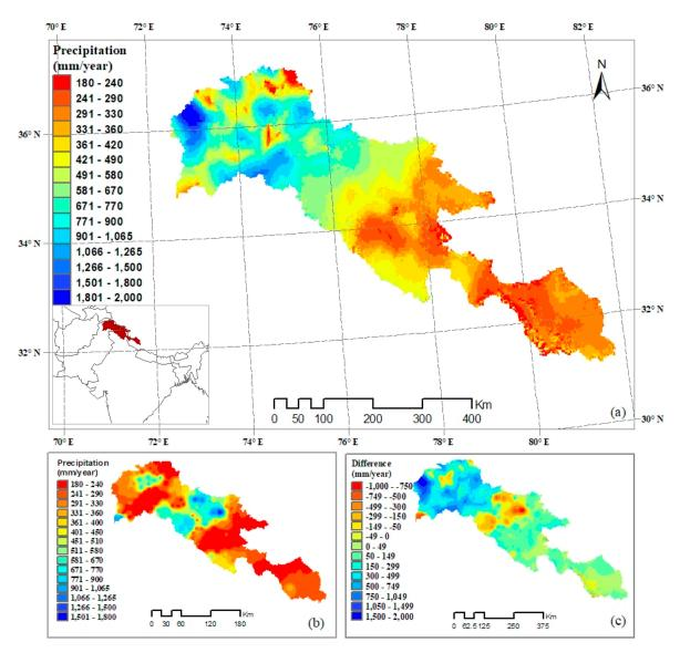
**Figure 3.** Generated gridded climate data set (1999–2008) for the UIB: (a) mean annual regionalized precipitation (mm), (b) mean annual observed precipitation (mm), (c) difference between regionalized and observed precipitation (mm).
