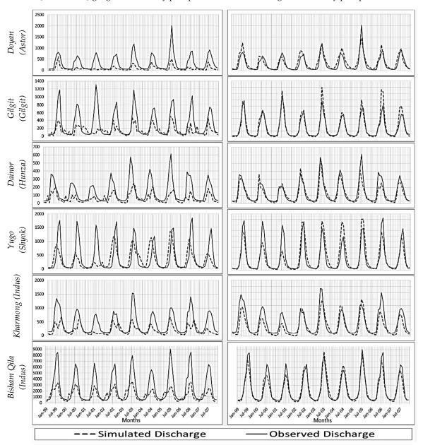
**Figure 4.** Comparison of SWAT-modelled flows with observed flows at different catchment outlets in the UIB when forcing the model with observed gauge station (**left** column) and corrected, regionalized (**right** column) precipitation.
