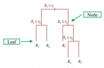
**Figure 1.** Decision tree example (adapted from Hastie et al. [58], p.306).  $X_j$  denote predictor variables. The tree has four internal nodes and five leaves (terminal nodes).  $X_j \le t_k$  and  $X_j > t_k$  correspond to the left and right branches of each internal split, respectively.  $R_i$  denotes the mean of the observations at leaf *i* [39] (p. 304).
