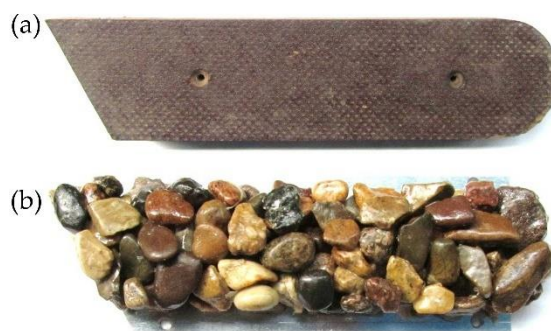
Figure 1. Top view on (a) the multiplex groyne model and (b) the gravel groyne model.
