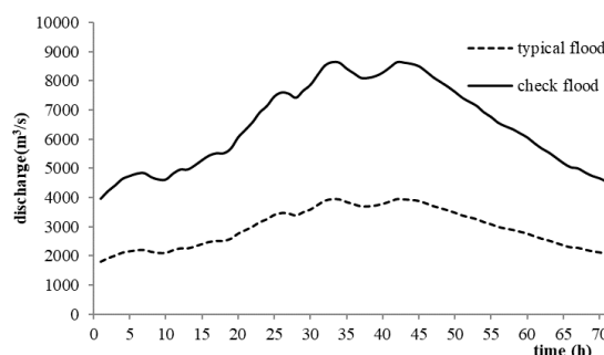
Figure 14. SJK dam check flood hydrographs and measured flood hydrograph in 1981.
