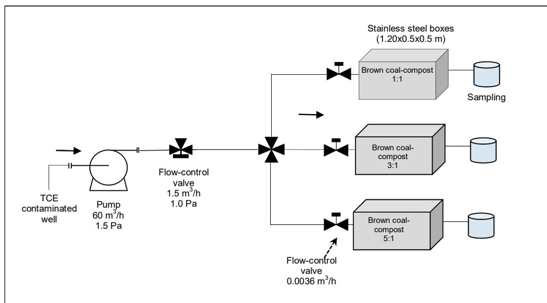
**Figure 2.** Schematic representation of the pilot brown coal-compost permeable reactive barrier (PRB) installation at the site.
