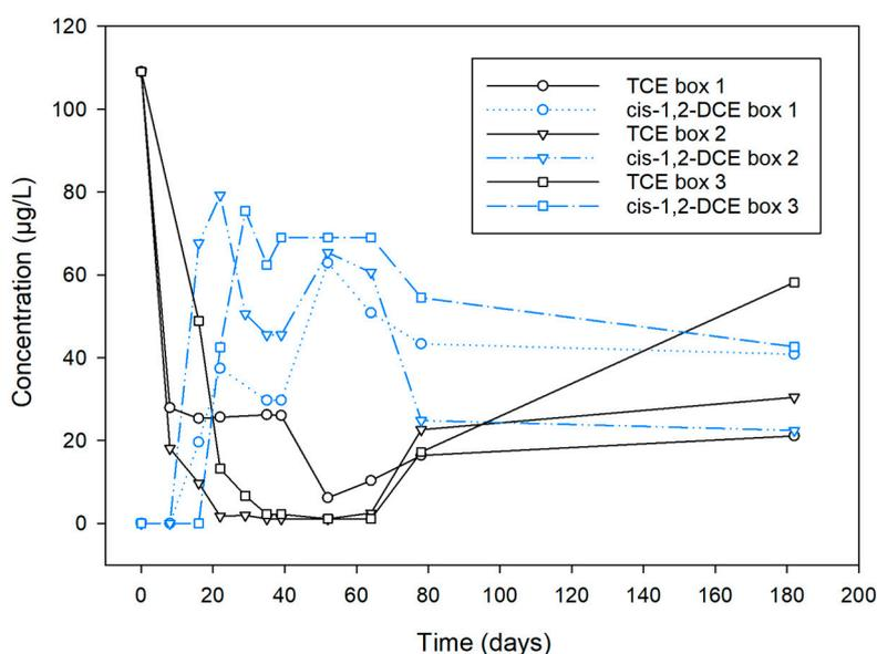
**Figure 4.** Concentrations of TCE and cis-1,2-DCE versus operation time of the experiments.
