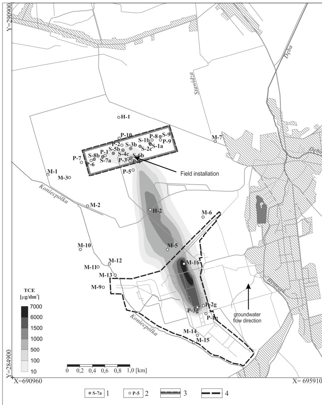
**Figure 1.** Overview map of the contaminated site including the location of metal-works factory, the affected waterworks and the estimated extent of the contaminant plume. Notation: 1—extraction wells; 2—piezometers; 3—waterworks area; 4—metal-works area.
