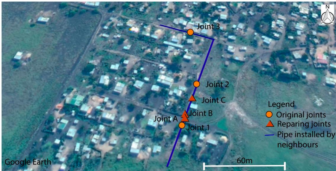
**Figure 7.** Location of joints in the pipe installed by the neighbors in Block Q11 (Map: Chitata, 2019).
