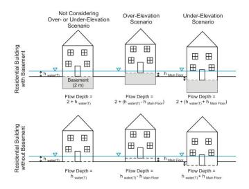
**Figure 3.** Flow depth estimation in the houses considering topographic over– or under–elevation with respect to the surrounding land, in the case of residential buildings both with and without a basement.
