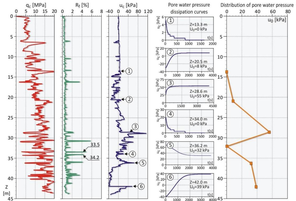
Figure 7. Identification of water conditions of sediments based on cone penetration test (CPTU) results.
