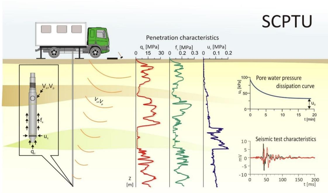
Figure 5. Principles of seismic piezocone testing.
