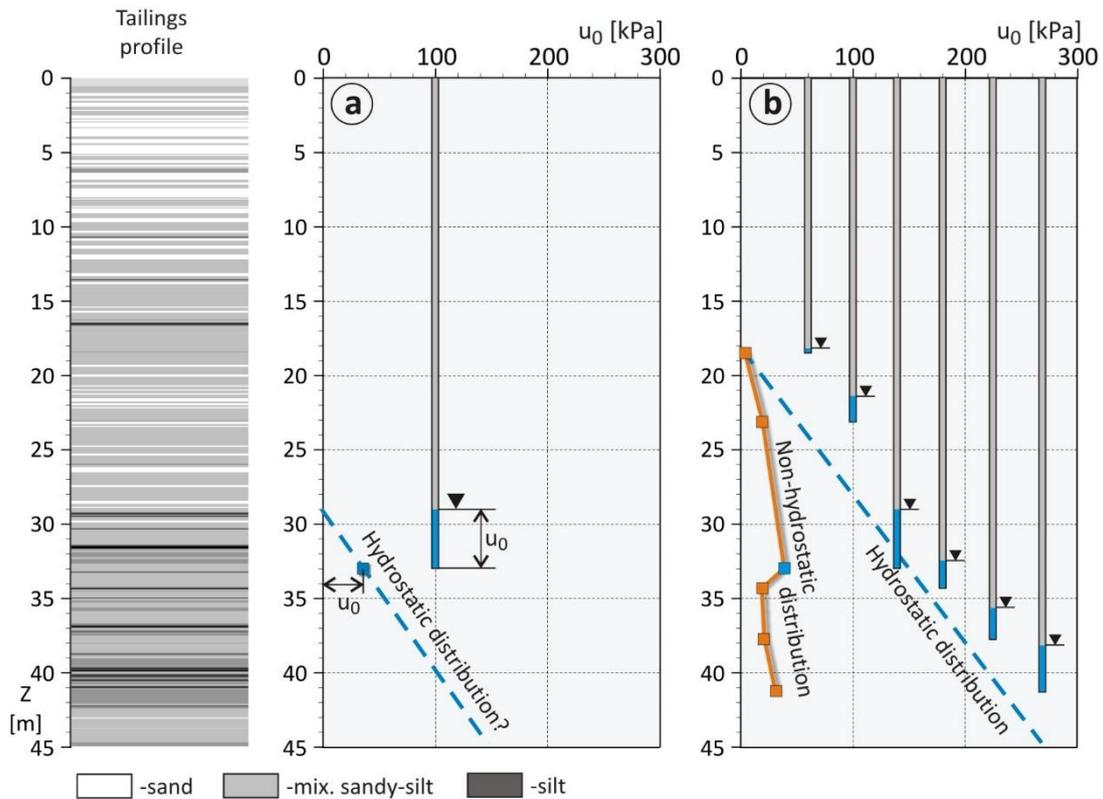
**Figure 6.** The comparison of the assessment of water conditions in sediments based on (a) single and (b) multiple piezometers readings.
