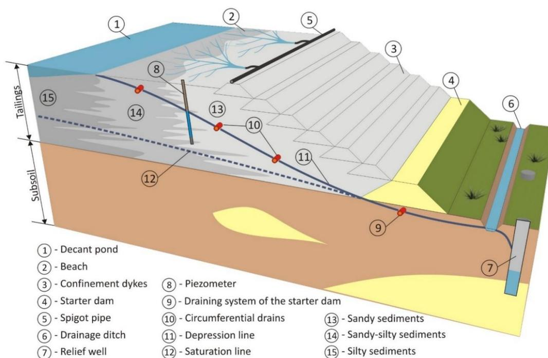
**Figure 4.** Schematic cross-section of ring dam and drainage system.
