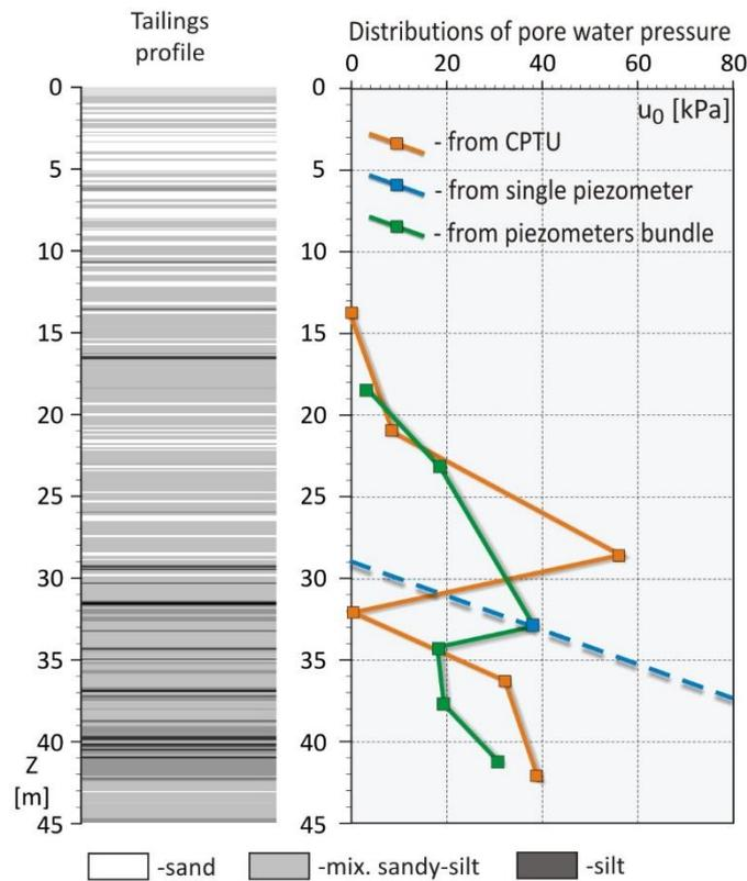
Figure 8. The comparison of water conditions in sediments with the piezometric methods and based on CPTU.
