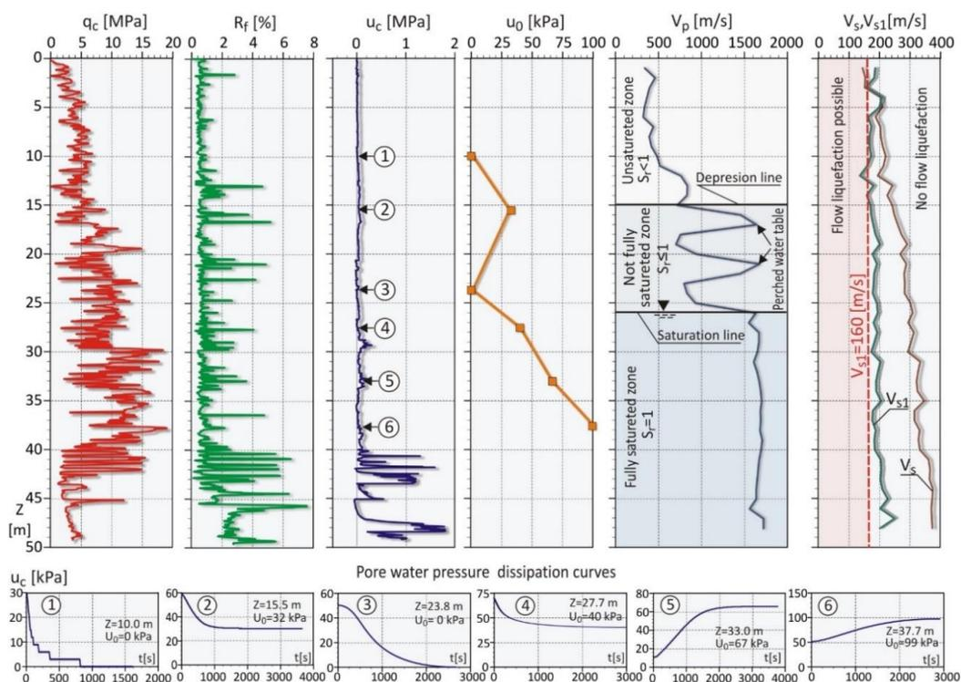
**Figure 9.** The complete assessment of water conditions in sediments with the seismic cone penetration test (SCPTU).
