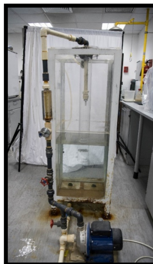
Figure 2. (a) Schematic of the confined plunging liquid jet experimental apparatus with the parts marked as follows: (1) Downcomer, (2) Nozzle (3) Water tank, (4) Rotameter, (5–9) Valves, (10) Pump, (11) Outlet, (12) Air tapping, and (13) Bubble meter. (b) Plunging Liquid Jet reactor built in the laboratory, as designed.
