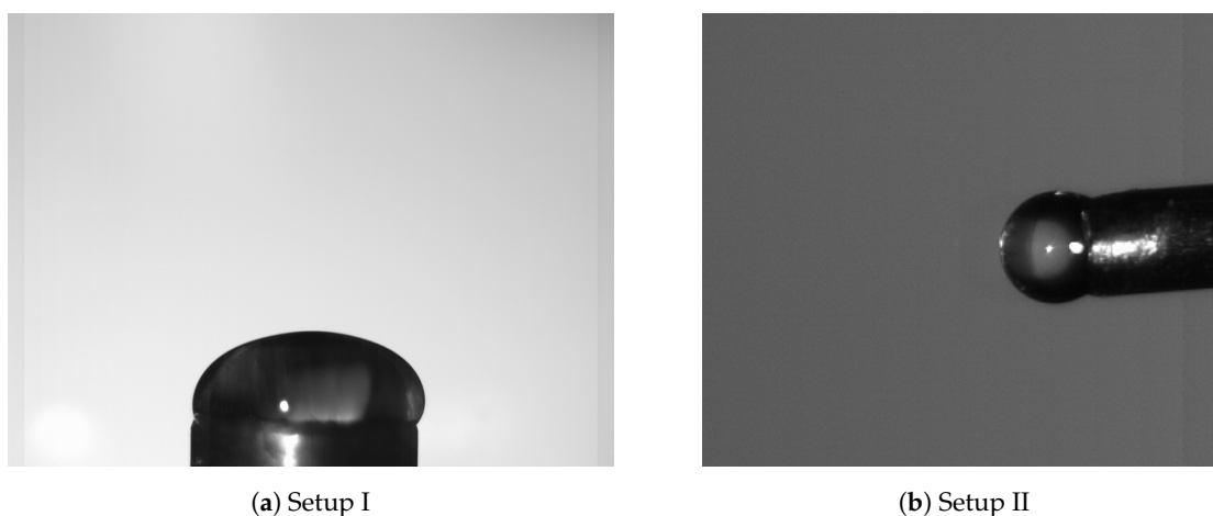
Figure 5. Photographs of initial droplets, just before the electric field was applied. (a) A droplet at vertical working electrode in setup I. (b) A droplet at horizontal working electrode in setup II. Photographs were exported from the record of the Olympus i-SPEED 720 high-speed camera using i-SPEED Software Suite [52].
