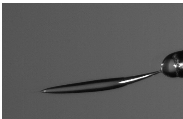
Figure 30. A spindle-like formation before the detachment from the mother droplet. The jet emanating from a tip of the spindle is visible on the left. The experiment was done in setup II with solution a0 at 22.0 °C and relative humidity 40%. Photographs were exported from the record of the Olympus i-SPEED 720 high-speed camera using i-SPEED Software Suite [52].
