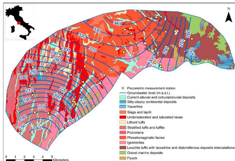
**Figure 4.** Groundwater level contour map of the southern Mounts Vulsini GWB and outcropping lithologies.
