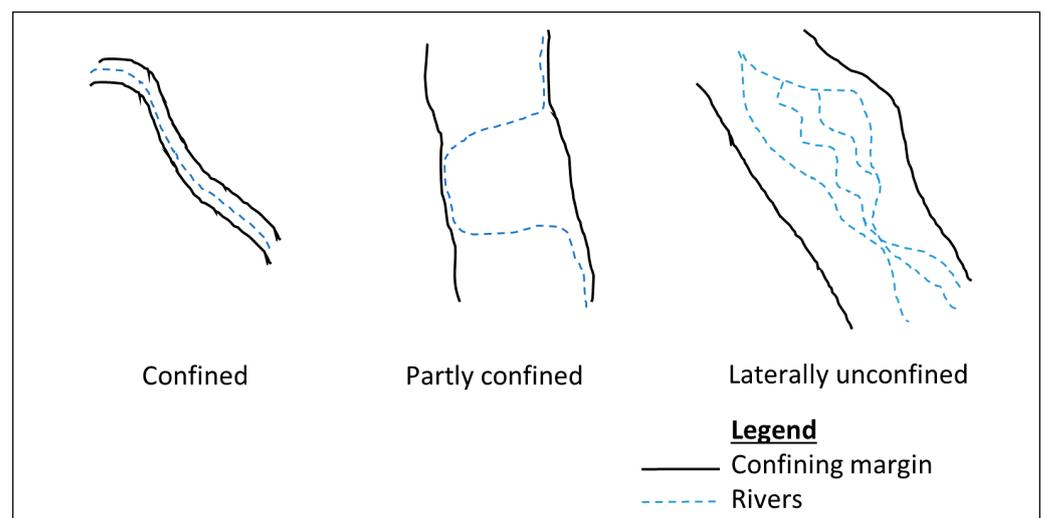
**Figure 2.** Different types of valley confinement modified from [10].
