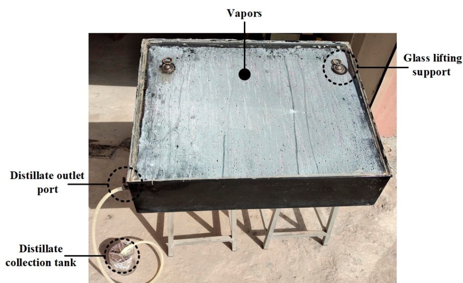
Figure 3. Single slope solar still experimental setup.
