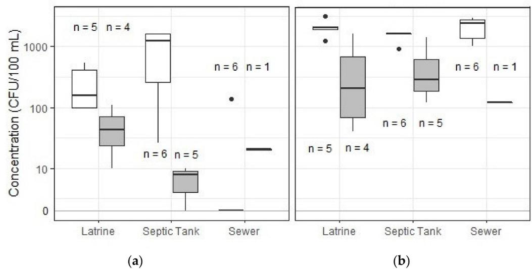
**Figure 12.** (a) *E. coli* and (b) TC concentration in water samples from households with a latrine/septic tank/small-scale sewer and a dug well/shallow well.
