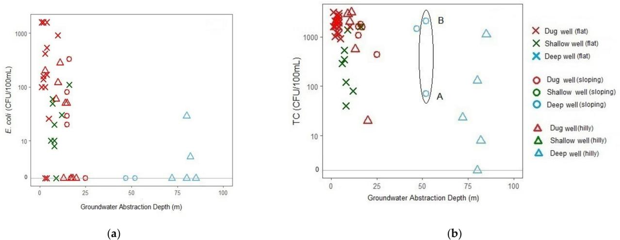
**Figure 9.** (a) *E. coli* and (b) TC concentration in water samples with different groundwater abstraction depths and well types. Water samples represented as A and B were collected from the same deep well but different households.
