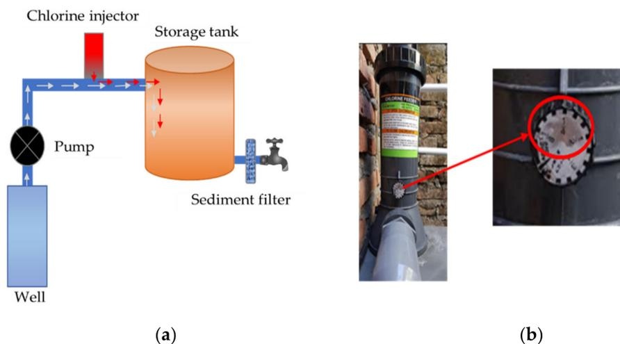
**Figure 4.** (a) Installation of chlorination system; (b) chlorine injector and controlling valve.
