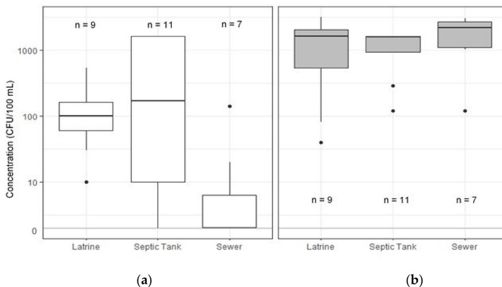
Figure 10. Distribution of (a) *E. coli* and (b) TC concentration in water samples at households using different types of sanitation facilities.
