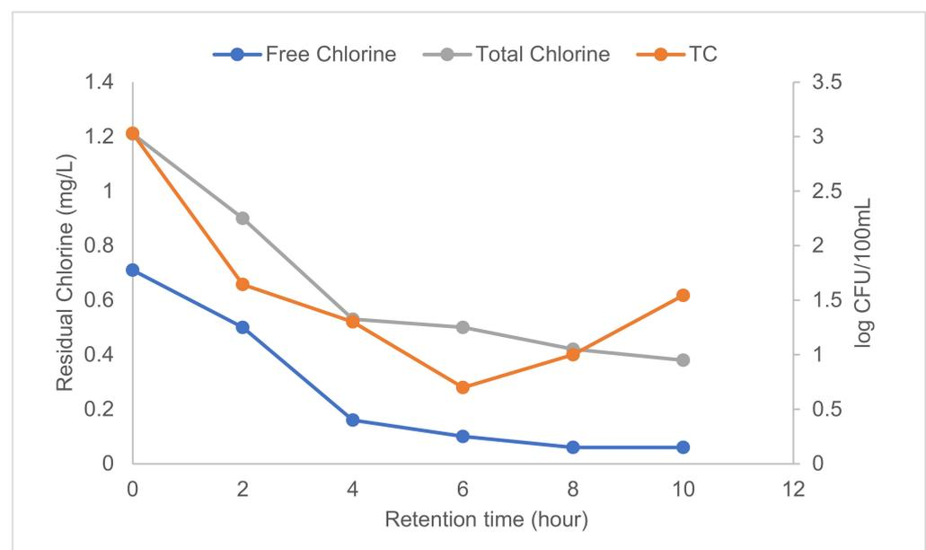
**Figure 13.** Change in concentration of TC, free chlorine, and total chlorine in treated water.
