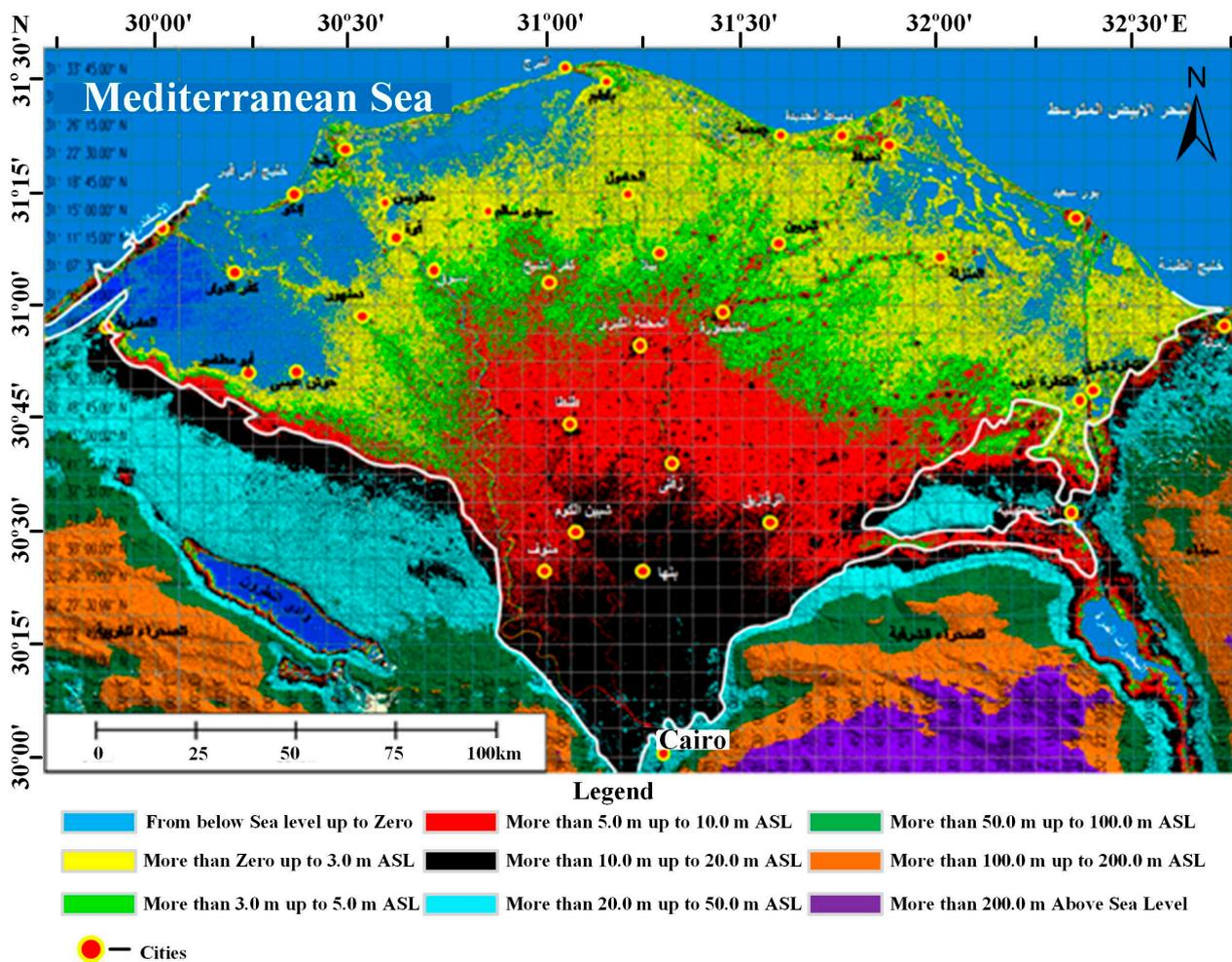
**Figure 5.** Coastal lowland of the Nile Delta: an extensive area (c. 7000 km<sup>2</sup>) ranging between 0–3 m above mean sea level is particularly vulnerable to the sea level rise.
