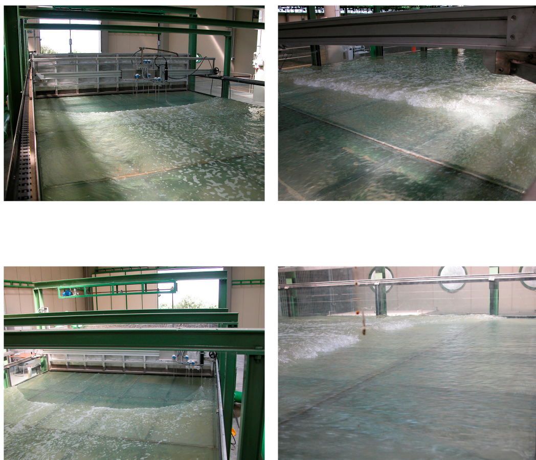
Figure 1. A hydraulic jump in the large channel of the LIC—Coastal Engineering Laboratory of the Polytechnic University of Bari, Italy. (See Video S1 in Supplementary Material).
