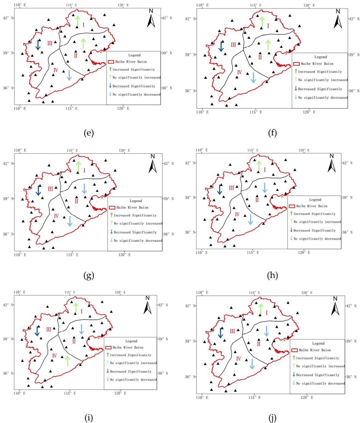
**Figure 6.** The Mann–Kendall (M–K) trend test results for the snowfall at the different levels in each zone in the Haihe River Basin (a) Average snowfall, (b) average snowfall days, (c) light snowfall, (d) light snowfall days, (e) moderate snowfall, (f) moderate snowfall days, (g) heavy snowfall, (h) heavy snowfall days, (i) snowstorm, (j) snowstorm days.
