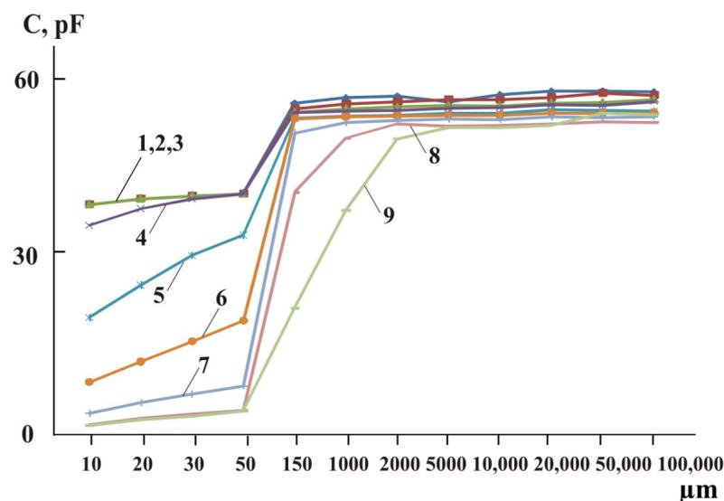
**Figure 2.** Dependence of the electrical capacitance ( $C$ , pF) of a sodium chloride solution with a concentration of  $1.5 \times 10^{-1}$  M on the distance between the capacitor plates ( $\mu\text{m}$ ) at different frequencies of reactive current: 1—1 kHz, 2—3 kHz, 3—10 kHz, 4—30 kHz, 5—100 kHz, 6—300 kHz, 7—1000 kHz, 8—3000 kHz, 9—10,000 kHz.
