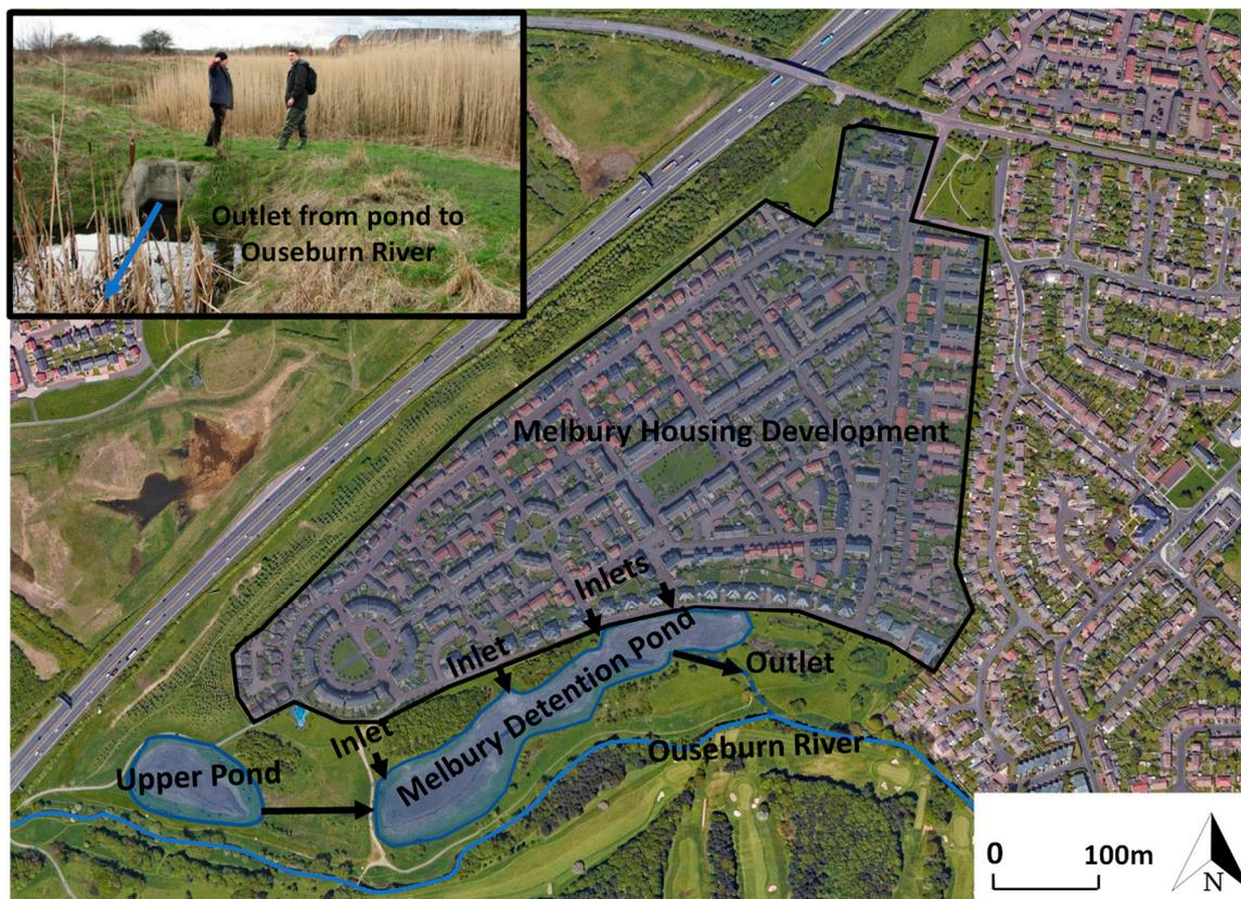
**Figure 6.** The Melbury housing development and detention pond within the Ouseburn catchment. The inset shows a picture of the pond outlet. Google Earth image (©Google, Digital Globe).
