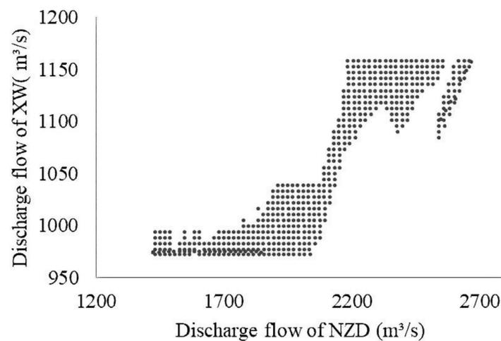
**Figure 14.** Optimized strategy combinations of hydropower stations during water supplement period (water supplement in March 1999).
