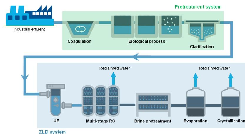
**Figure 1.** Typical processes to achieve zero liquid discharge (ZLD) in management of industrial effluent.
