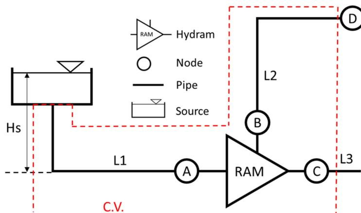
**Figure 1.** Hydrum basic components. Nodes A, B, and C refer to the connections of the drive pipe (L1), the discharge pipe (L2), and the waste valve, respectively. L3 refers to the pipe exiting the waste valve, node D refers to the uphill consumer and  $H_s$  denotes the upstream head. In the following equations,  $Q_i$  refers to the flow at pipe  $i$  in CMH, while  $H_j$  refers to the head at node  $j$  in meters.
