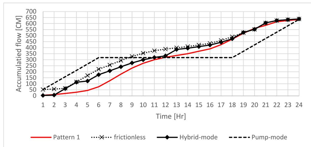
Figure 7. Accumulated Flows at the storage tank for case study 02.
