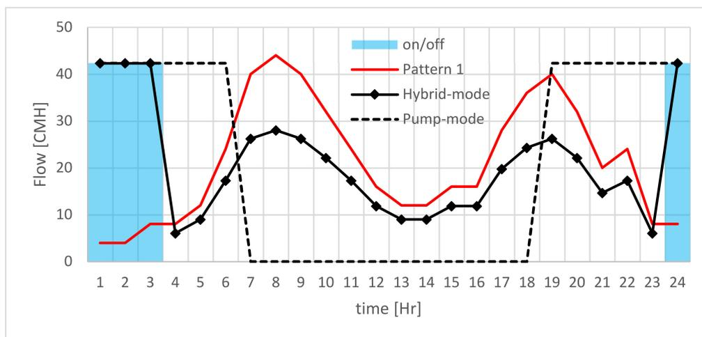
Figure 3. Storage unit inflows-outflows for case study 01 during the simulation period.
