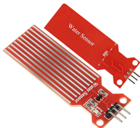
Figure 4. Water sensor used in [93], Courtesy of the Shenzhen Ke Zhi You Technology Co., Ltd., China.
