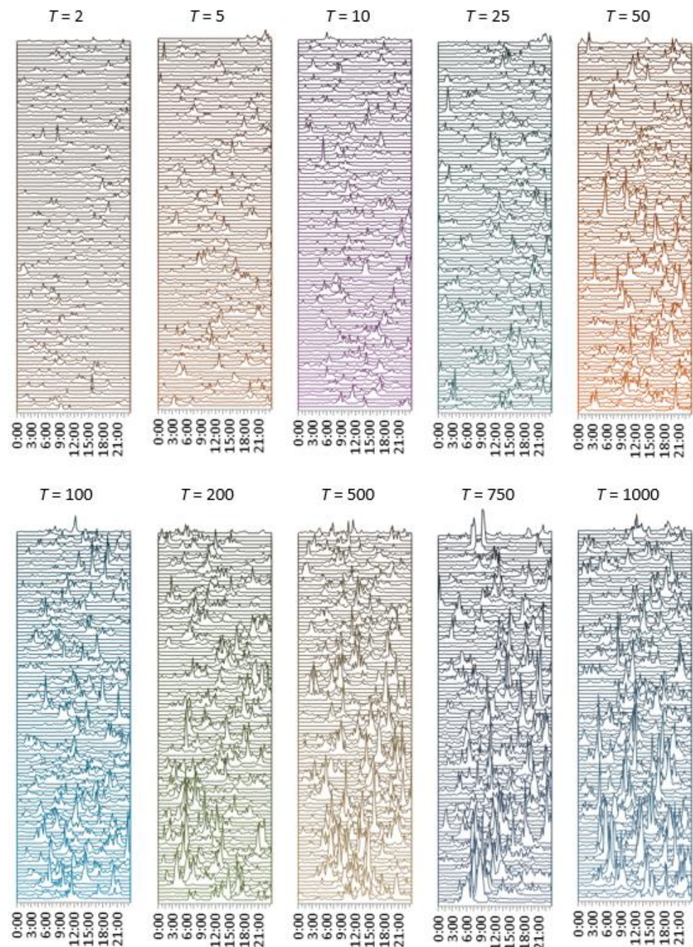
Figure 4. Synthetically generated 24 h design hyetographs (time interval 15 min), grouped by return period T (years) (100 synthetic hyetographs per T ).
