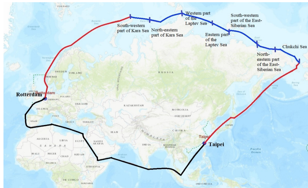
Figure 3. Routes along the Europe sea route (black) and Northeast Passage (red and blue). The Russian government zoned the Northeast Passage into seven areas (blue), which from east to west are the Chukchi Sea, North-eastern part of the East-Siberian Sea, South-western part of the East-Siberian Sea, Eastern part of the Laptev Sea, Western part of the Laptev Sea, North-eastern part of the Kara Sea, and South-western part of the Kara Sea.
