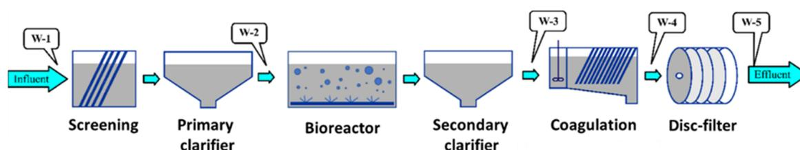
**Figure 1.** Sampling points and typical wastewater treatment process.
