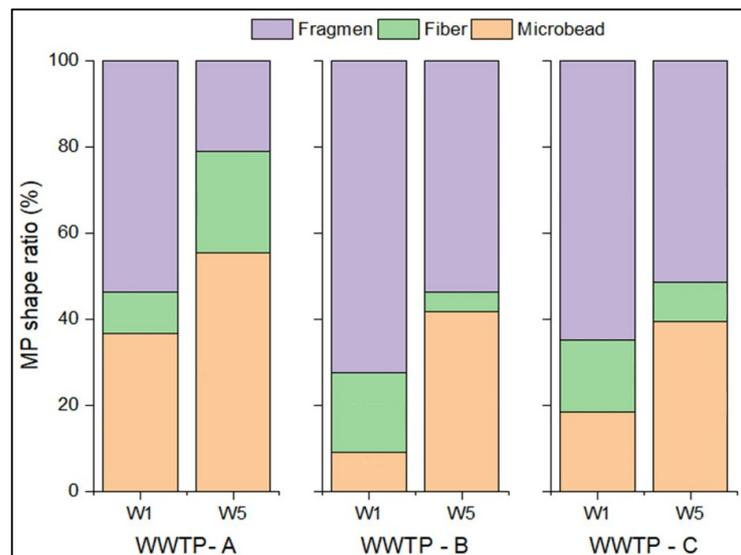
Figure 4. Comparison portion of microplastic shape between influent (W1) and effluent (W5).
