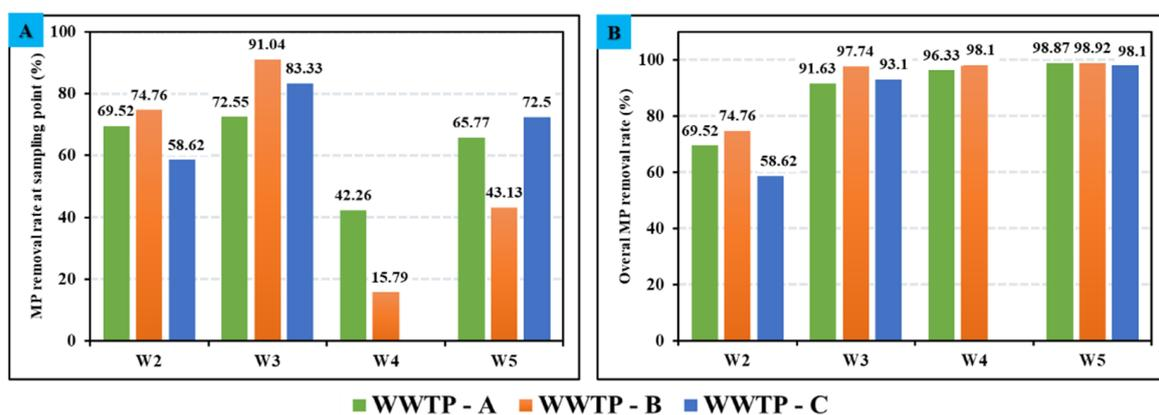
**Figure 2.** Removal of microplastic in different treatment processes. (A) Percentage of microplastics removed at sampling point; (B) Overall percentage of microplastic removal.
