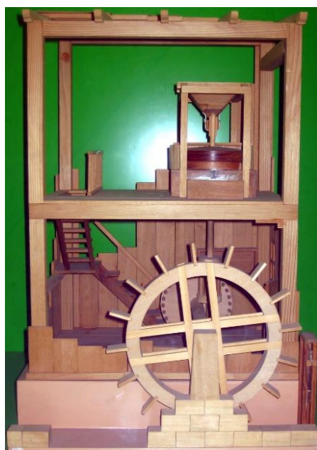
Figure 12. Reconstruction of a grain-mill following the principles of Vitruvius (ca 80–15 BC). The undershot waterwheel powered the gear mechanism (lower floor) and thus induced the millstone (upper floor) to function ( https://en.wikipedia.org/wiki/Public_domain , assessed on 1 September 2022).
