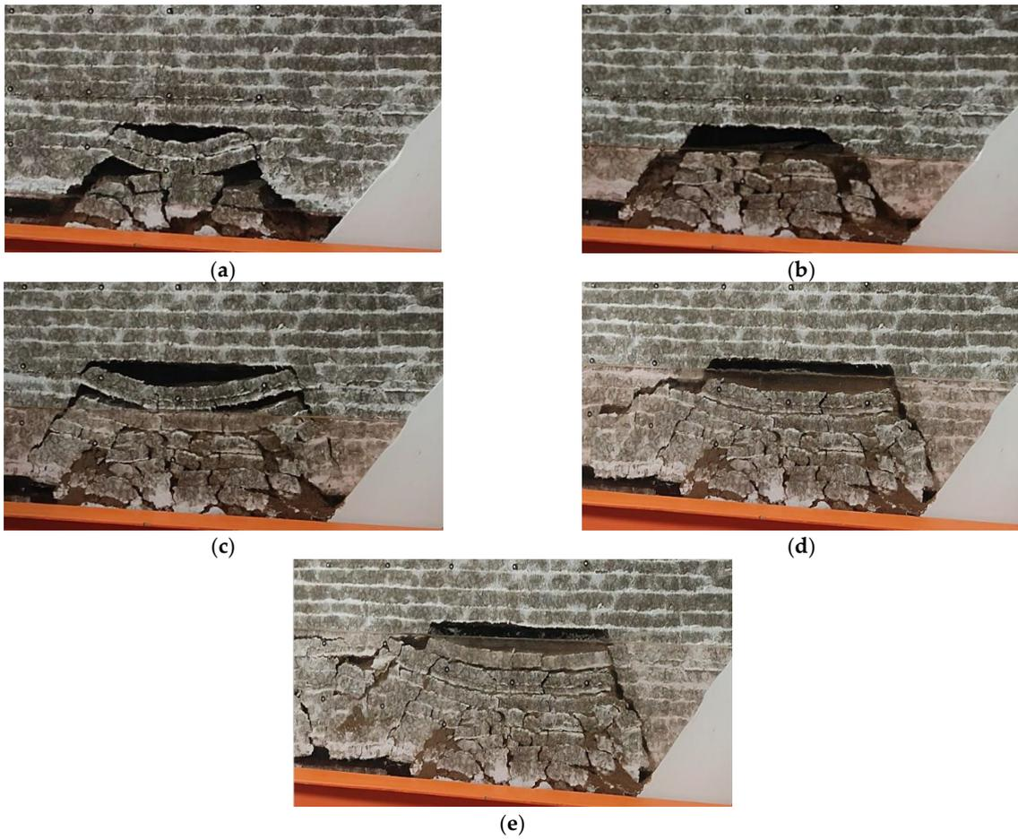
**Figure 9.** Evolution of overburden destruction on the right side in coal pillar corrosion stage affected by water immersion in the strip goaf. (a) Water starts to inrush in goaf. (b–e) First, second, third, and fourth instances of shear damage of coal pillar, respectively.
