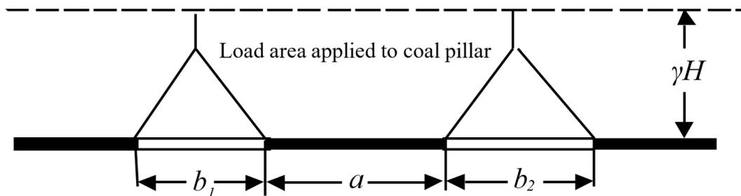
Figure 13. Wilson’s coal pillar load calculation method.
