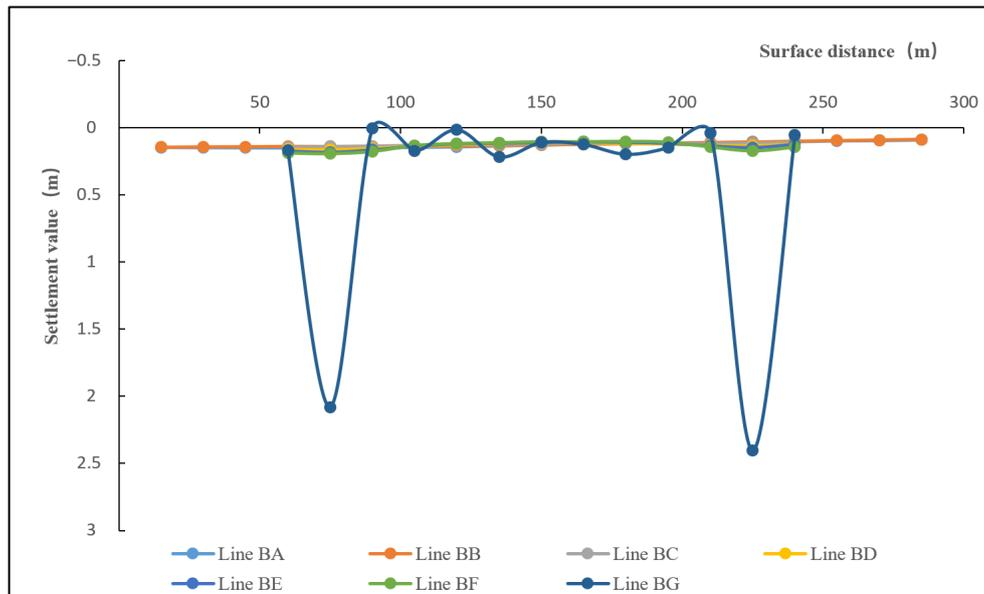
**Figure 7.** Overburden subsidence curves of strip mining.
