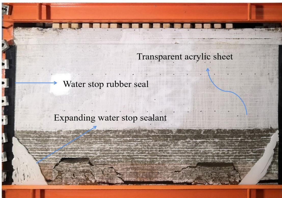
**Figure 8.** Model sealing effect.
