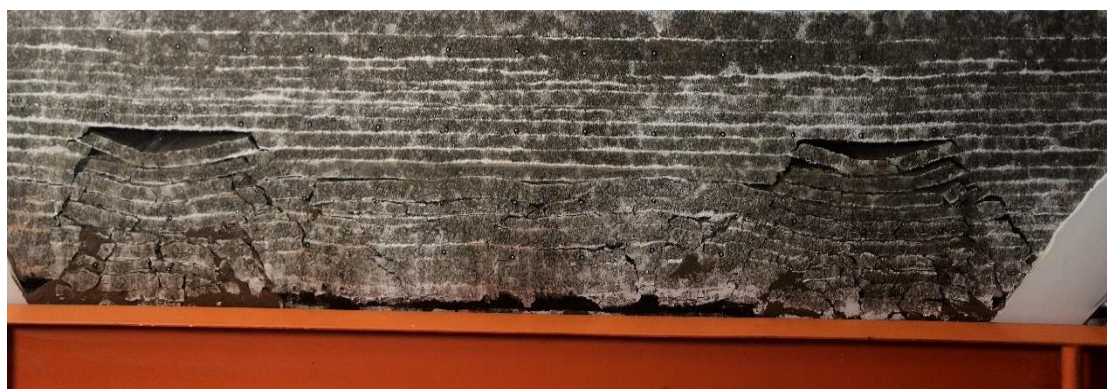
Figure 11. Overburden damage pattern of coal pillar destabilization affected by water immersion in the strip goaf.
