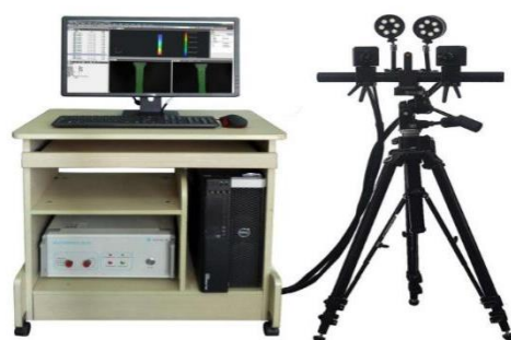
Figure 5. Non-contact video strain displacement precision measurement system.
