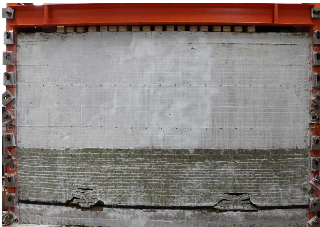
Figure 6. Overburden failure of strip mining.
