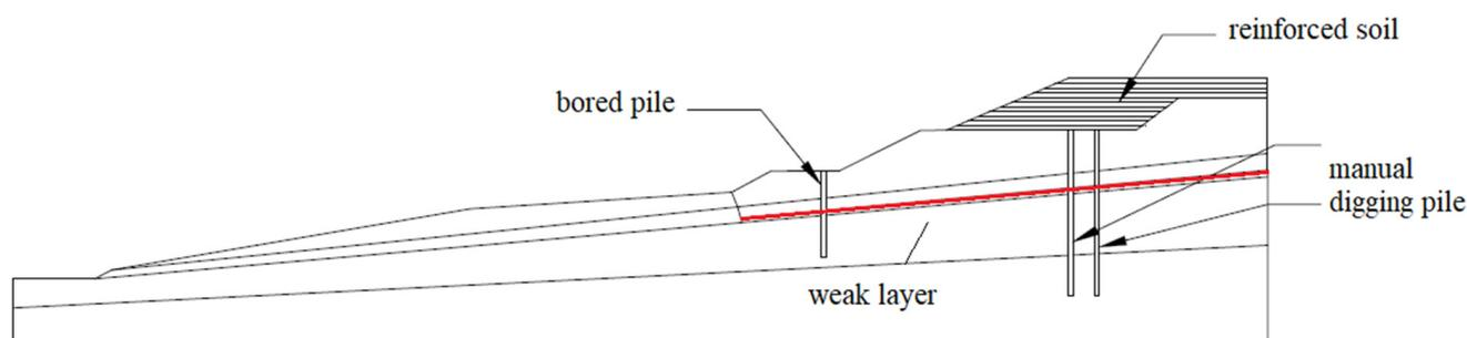
**Figure 14.** Final reinforcement scheme of slope.
