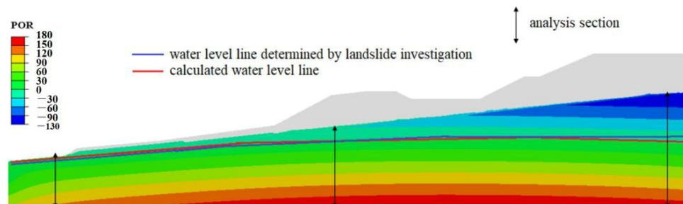
Figure 6. Overall pore pressure of slope.
