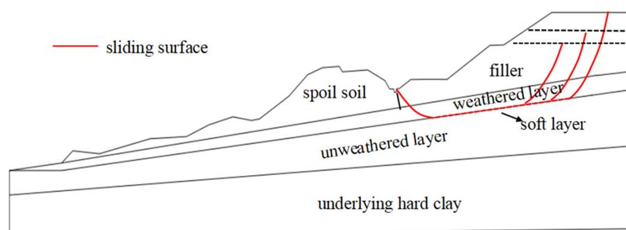
**Figure 13.** Influence of different unloading heights on slope sliding surface.
