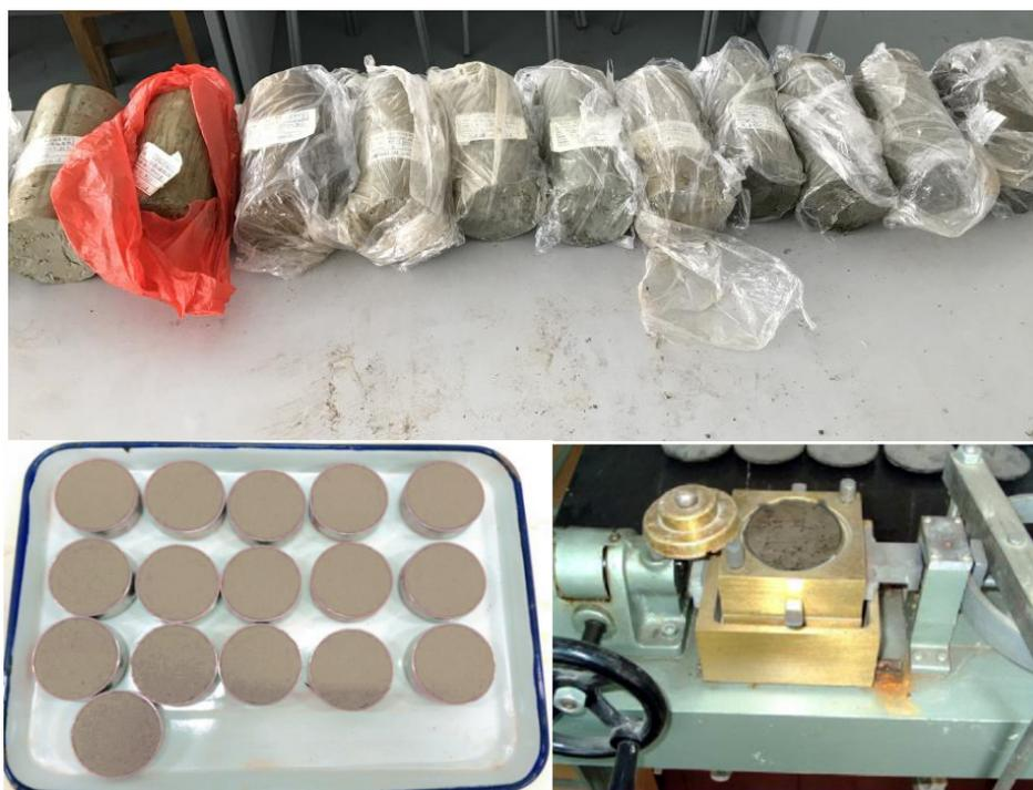
**Figure 1.** Strength test of the undisturbed soil sample.
