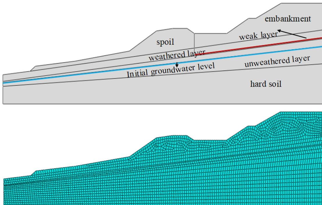
Figure 4. Basic model of slope.
