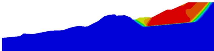
**Figure 11.** Potential sliding surface of slope ( $F_s = 0.97$ ).
