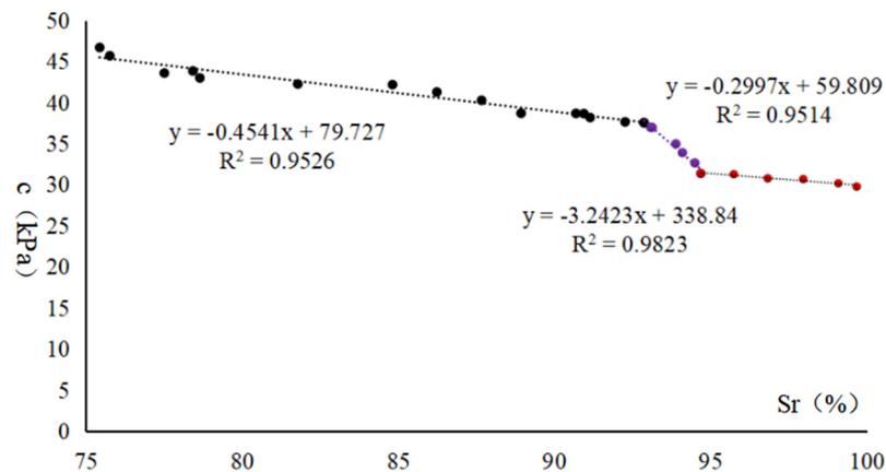
Figure 2. Relationship between humidity and cohesion c.
