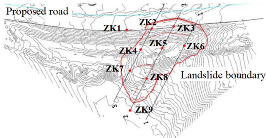
Figure 9. Scope of landslide.
