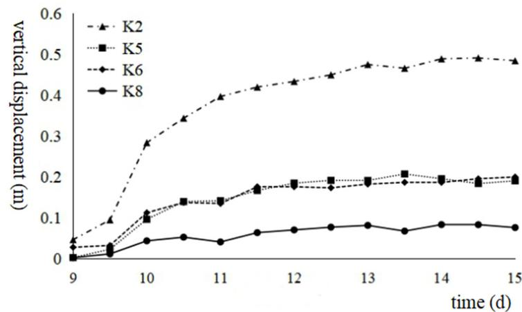
Figure 10. Vertical displacement of slope monitoring point.
