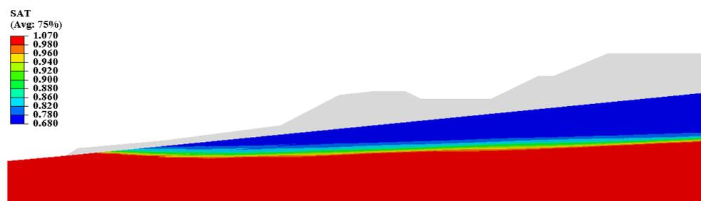
Figure 5. Overall saturation of slope.
