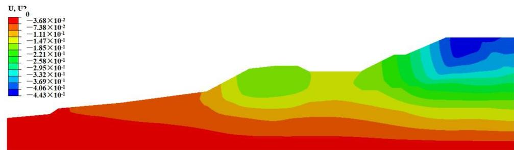
Figure 8. Vertical displacement of slope.
