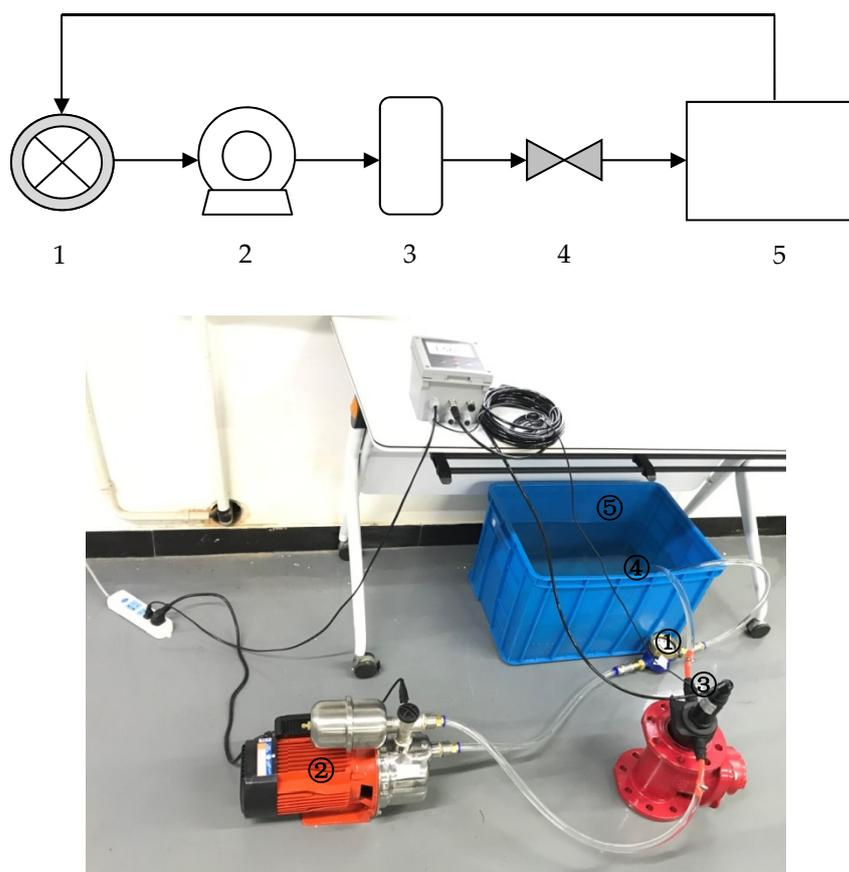
**Figure 1.** Schematic diagram and actual picture of the experimental setup. 1. Water meter; 2. Variable frequency pump; 3. Chemitec in-line turbidity meter (including temperature sensor); 4. Ball valve; 5. Water tank.
