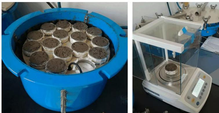
**Figure 4.** Test device for the pressure film meter method.
