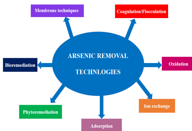
Figure 4. Various arsenic removal technologies.
