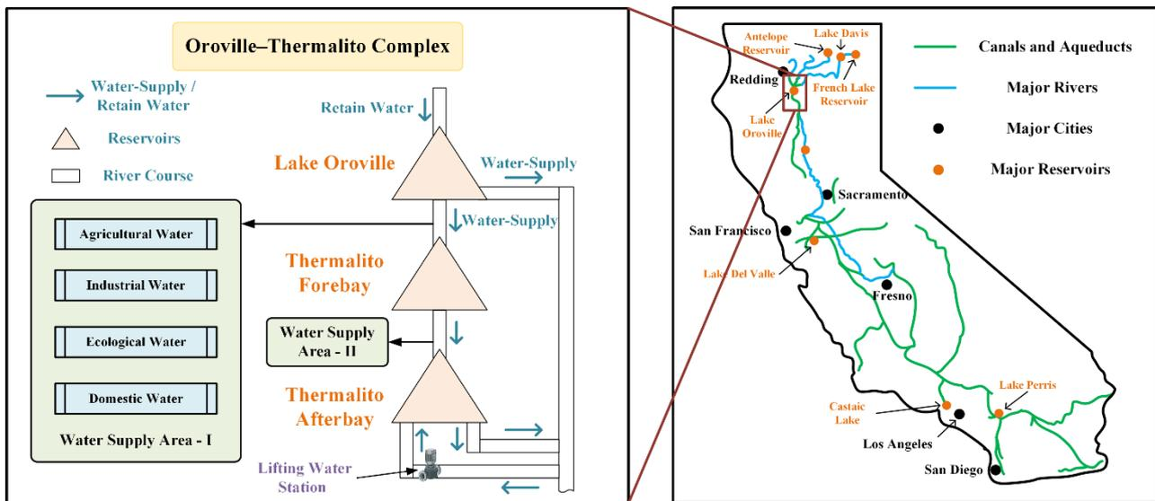
**Figure 2.** Topological structure diagram of cascade reservoir system in the Oroville–Thermalito Complex.
