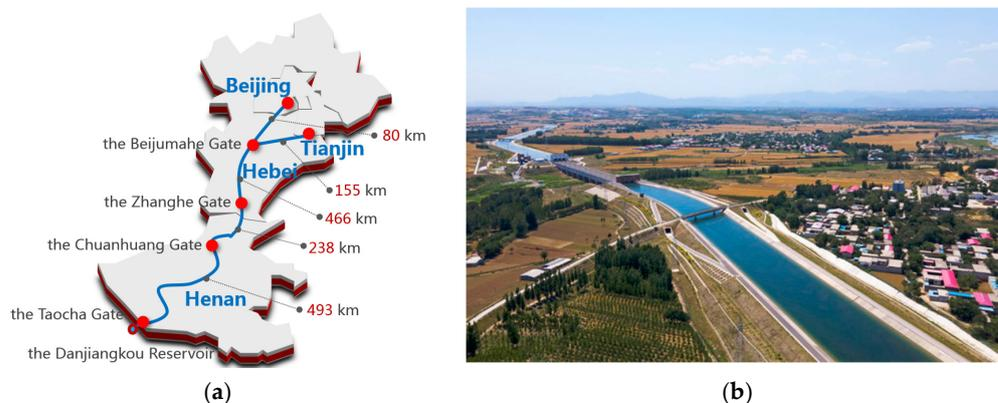
**Figure 1.** Main canal of the middle route of the South-to-North Water Diversion Project: (a) general layout and (b) canal and crossing water-conveyance structures.
