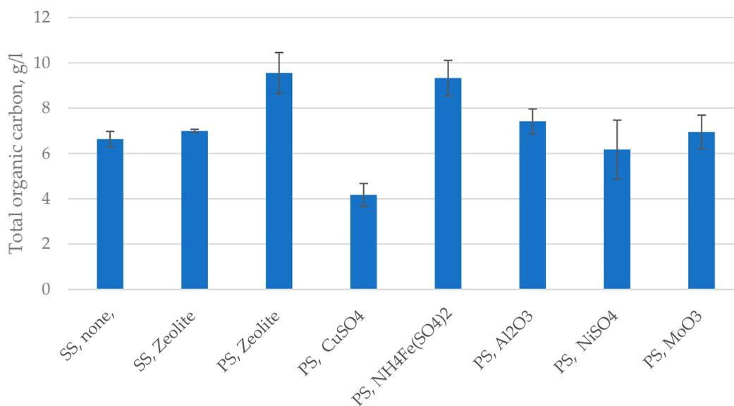
**Figure 4.** Dependence of HTL-AP contamination by organic compounds on the type of sludge and process conditions.
